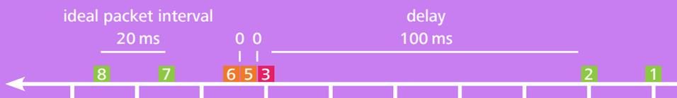
Schematic packet flow of impaired voice transmission by network
